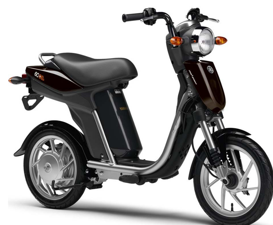
Fig.3. Yamaha EC-03 is a LETW with range of 45 km, maximum speed of 45 kmph and weighs only 56kg (in comparison, a 50 cc scooter weighs nearly 90kg)
