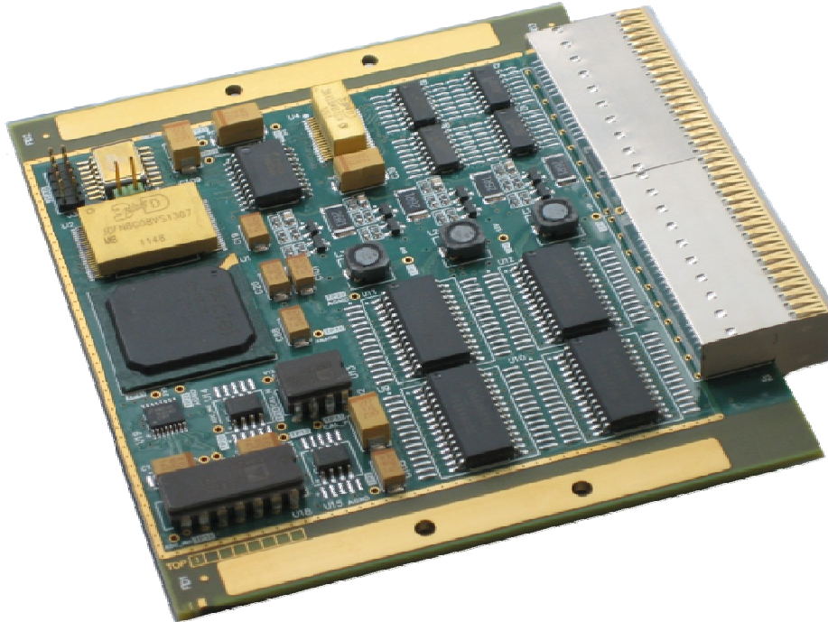
Figure: MASCOT IO board (based on commercial quality components)
