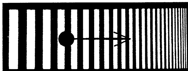
Fig.1.1.7. a. Schematic drawing of a spherical particle passing across a variable frequency grid [1.32].
