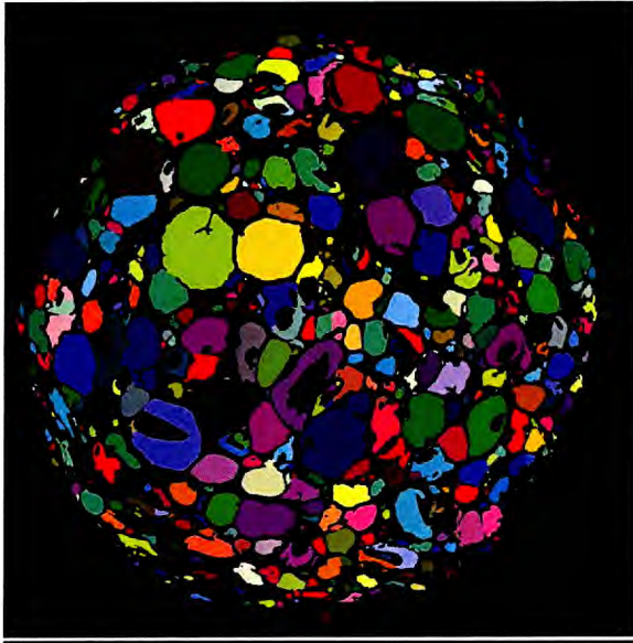
Figure 3.30: 2-D section through porous extrudate showing segmented pores in different colours (i.e. different pores are different colours) with solid and external air being black.
