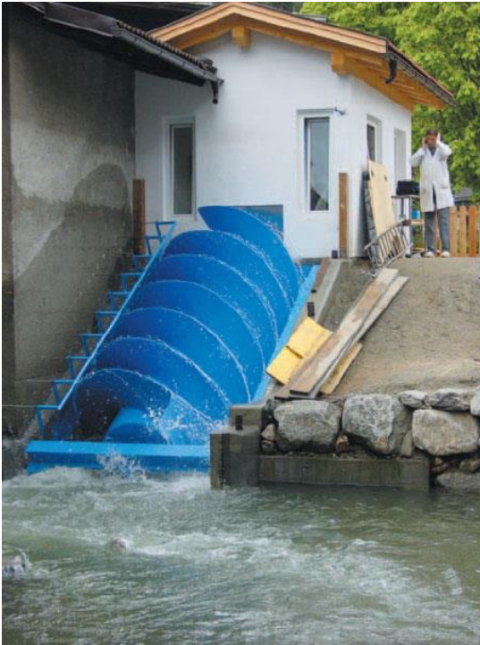
Helical or Alden turbine (DOE-EPRI 2011)
