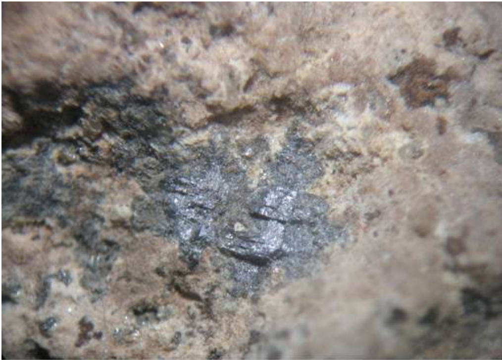
Fig. 14 - Enlarged (X 40) disseminated Galena in Miocene carbonates
