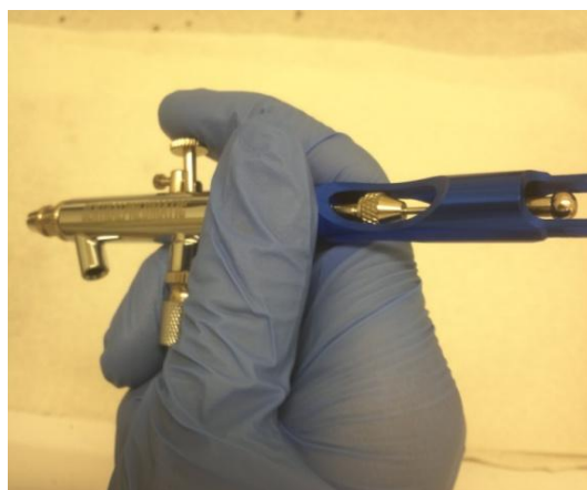
Figure 3.9 - The airbrush spray gun used for imparting HFGO inks onto the desired porous/non-porous substrates.
