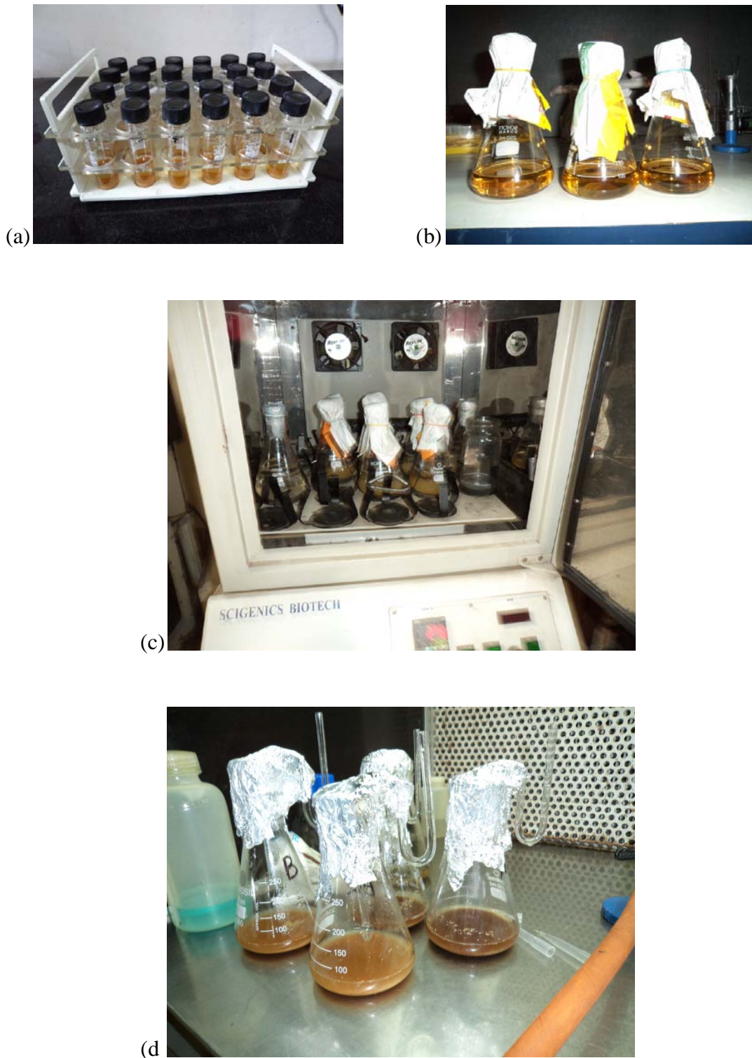
Figure 4.5 – Pretreated samples preparation for enzymatic hydrolysis and fermentation. (a): Pretreated samples in serum bottles for enzymatic hydrolysis. (b): Culture media and glassware set for autoclaving. (c): Cultured media in a shaking incubator. (d): Pretreated samples in fermentation flasks (air tight) with U-tube glass ready for incubation at 32 °C.
