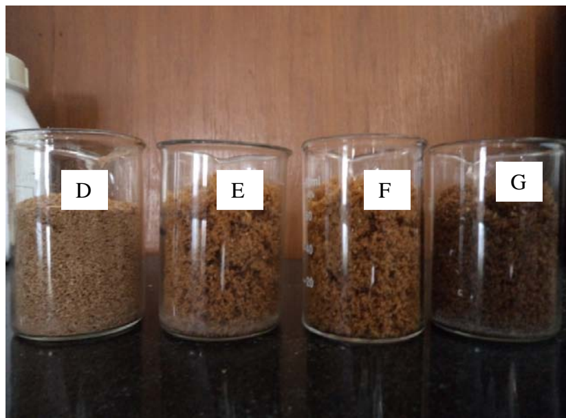
Figure 3.4 – ((a) and (b)). Slurry and solid fraction of pretreated biomass. (A): Slurry before pretreatment. (B): Slurry after pretreatment. (C): Slurry after neutralization. (D): Raw dry biomass. (E) and (F): Wet biomass after APO pretreatments at 120 °C and 135 °C respectively. (G): Wet biomass after APO pretreatment at 150 °C.
