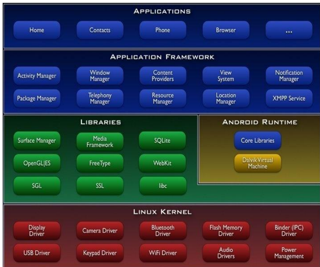
Figure 4.1: The Android Platform Architecture (Burnette, 2010)
