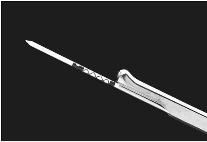
Fig. 3. Interstitial laser applicator, low-OH quartz glass fiber 600 \mu\text{m} , applicator 1.8 mm in diameter, 2 cm in length, 160°-cone shape radiation pattern (in air or water).
