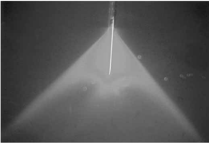
Fig. 1. ITT light guide, quartz glass fiber 600 \mu\text{m} , applicator 1.9 mm in diameter, 2 cm in length, 90°-cone shape radiation pattern (in air or water).
