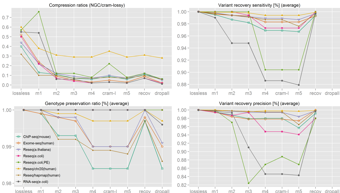
Figure 4.4: Evaluation data. The upper-left figure compares the compression ratios of the different modes for the used evaluation data sets (cram-l refers to the used cram-lossy mode). The absolute byte sizes and the compression ratios of the decompressed BAM files can be found in Appendix A. Note that the Reseq/q/chr20 (human) BAM files are less compressible as they contain large sections of optional BAM tags (see Appendix A). The figures on the right side show the variant recovery precision and sensitivity averaged over the data we obtained by applying two different variant-calling tools (GATK and SAMTOOLS). We omitted the data for the “drop all” mode in these two figures for readability as the corresponding values would require a much larger scale. The lower-left figure shows how many of the re-found variants (i.e., the true positives) did not change their predicted genotype classification, either from homozygous to heterozygous or vice versa. All absolute data values and the used command-line parameters are given in Appendix A. Please note the differing scales of the y-axes in the four figures.
