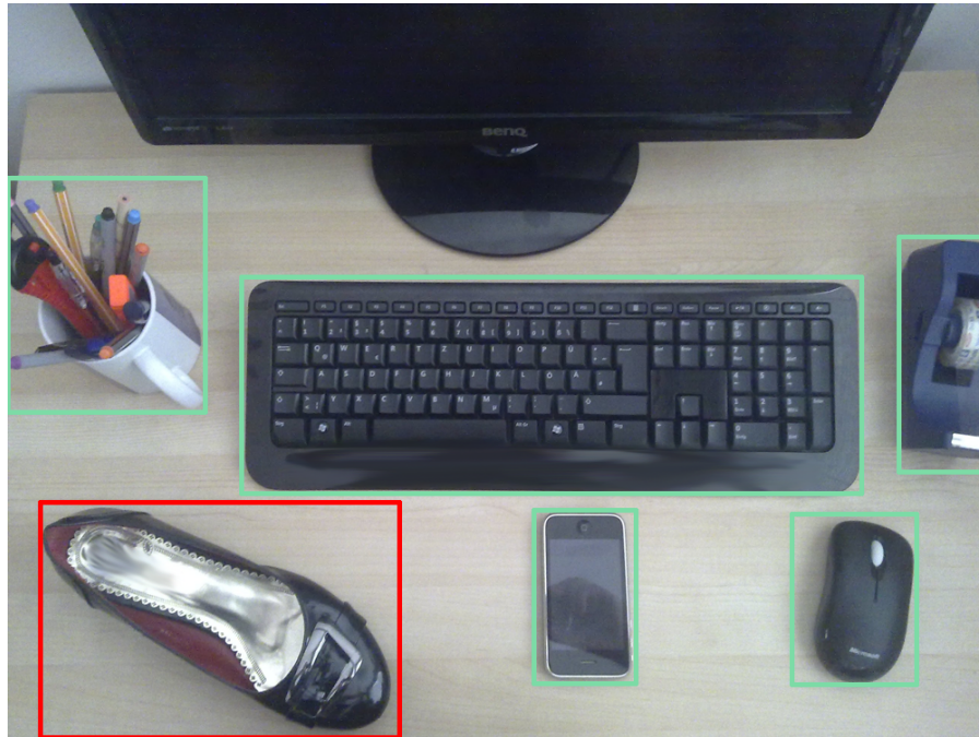
Figure 4.17: Objects with green borders have been identified and exist in the database of table objects, but the shoe, which has a red border, has not been identified before and does not exist in the database. Since the computer monitor position is fixed, it has been assumed to be part of the table.
