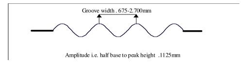
Figure 2. Parameters of the sinusoidal waveform.
