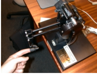
Figure 2: The Phantom haptic device
