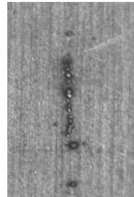
Fig. 2. Entry (left) and exit (right) side at 800 Hz, 20 mm/s. There is no cut, but spattering.
