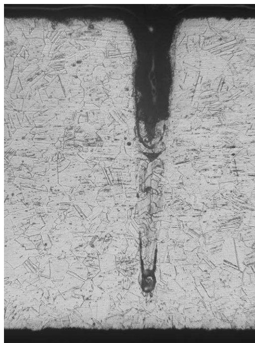
Fig. 3. Cross section of the kerf at 800 Hz, 20 mm/s laser setting (no cut).
