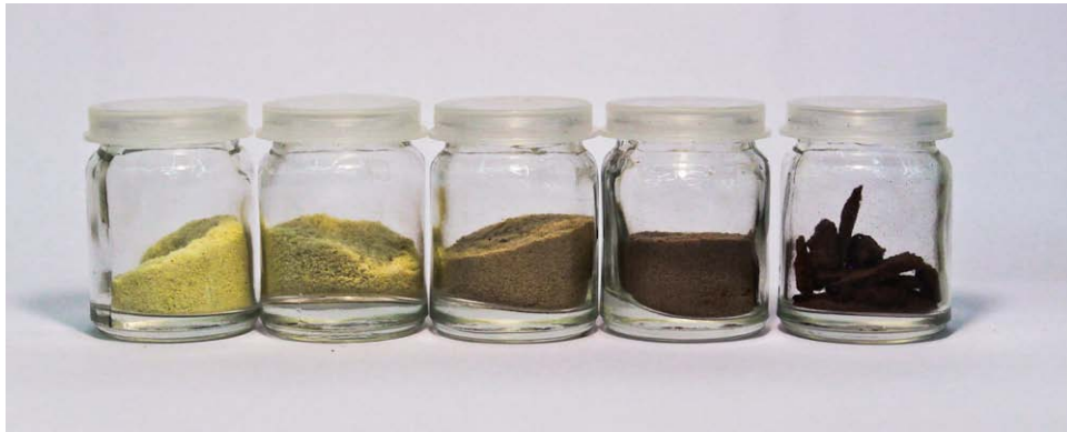
Fig. 4 Wood particles impregnated with phenolic resin solutions of different solid content; concentration is 0.5, 1, 3, 5, and 10 wt%, respectively, and increases from left to right.
