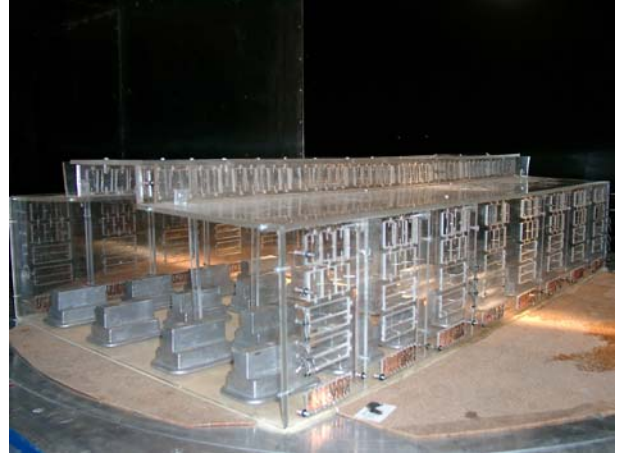
Fig. 2 The plexi-glass 1:80 scale model of the workshop on a rotary table in the wind tunnel
