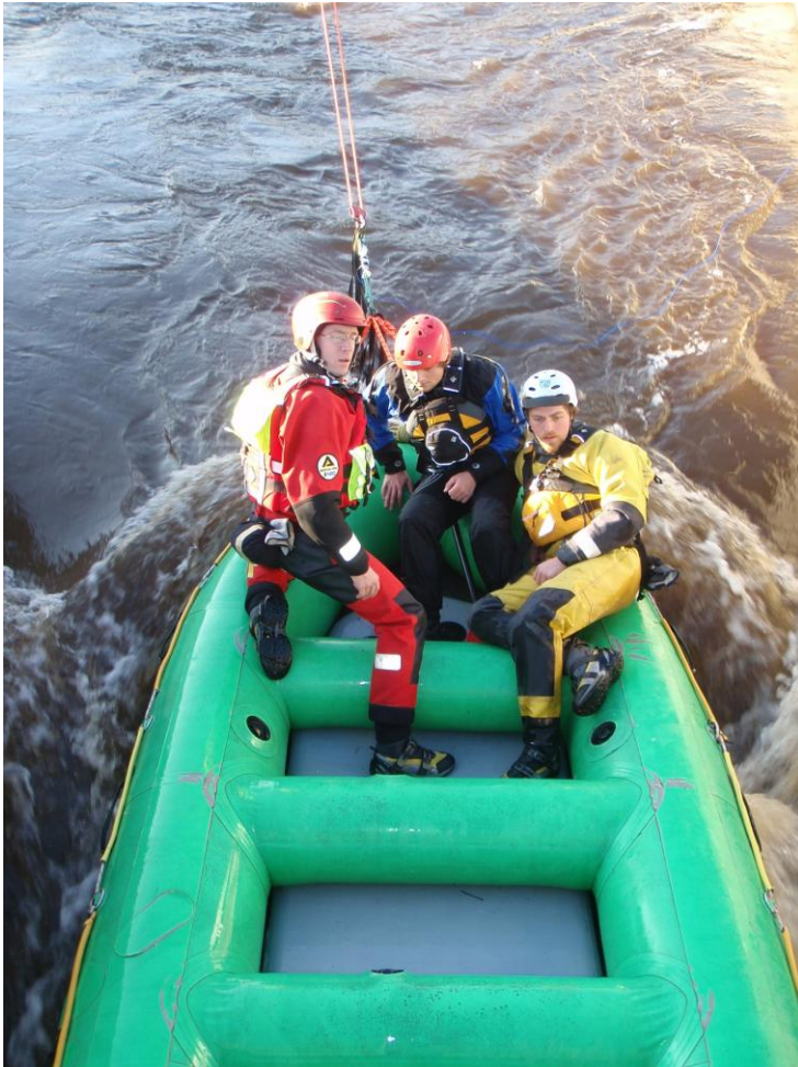
Figure 4. Boat set up for Bow Trim. Note three technicians placed towards the bow.
