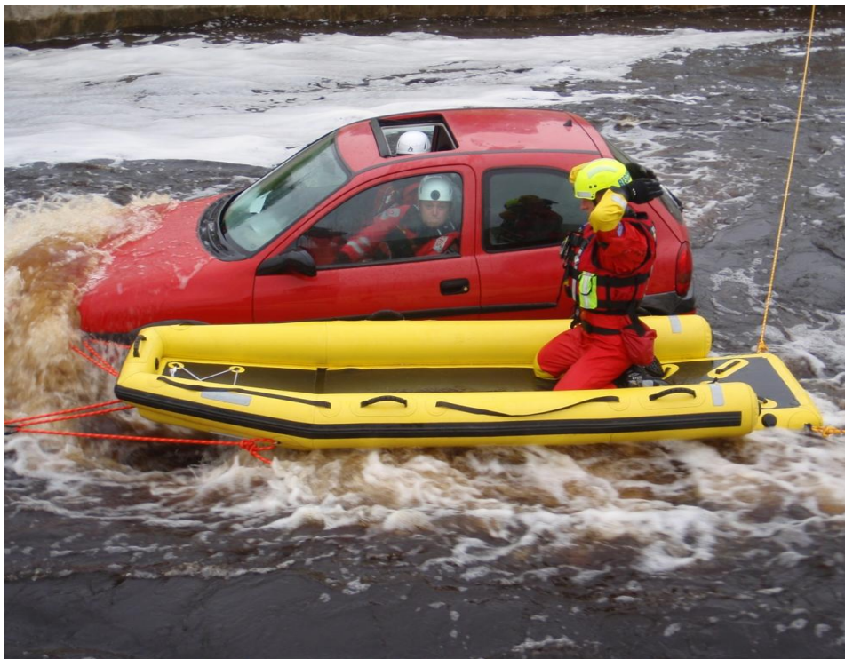
Figure 4. An MFC Rescue Sled™ shown during a rescue from vehicles in water training class. The car is aligned with the direction of the current (bonnet facing up-stream) and the rescuer is using hand signals to indicate that the sled should be moved rearwards. Note the smaller tubes (sponsens) and reduced carrying capacity of the sled.
