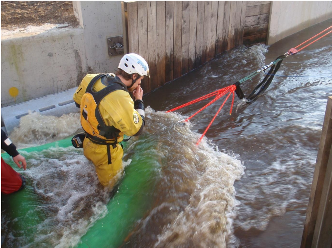
Figure 6. The bow is deliberately swamped during the testing of the Worst Case Event. The Technician is considering the implications of severing one of the anchor legs under these conditions.
