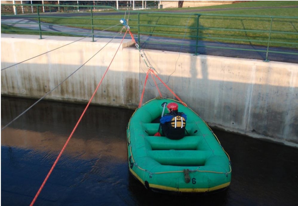
Figure 3. A Eurocraft raft positioned in the testing channel. Note the construction with large tubes (sponsens) contributing to the enhanced stability of the craft and the potential for carrying multiple passengers.
