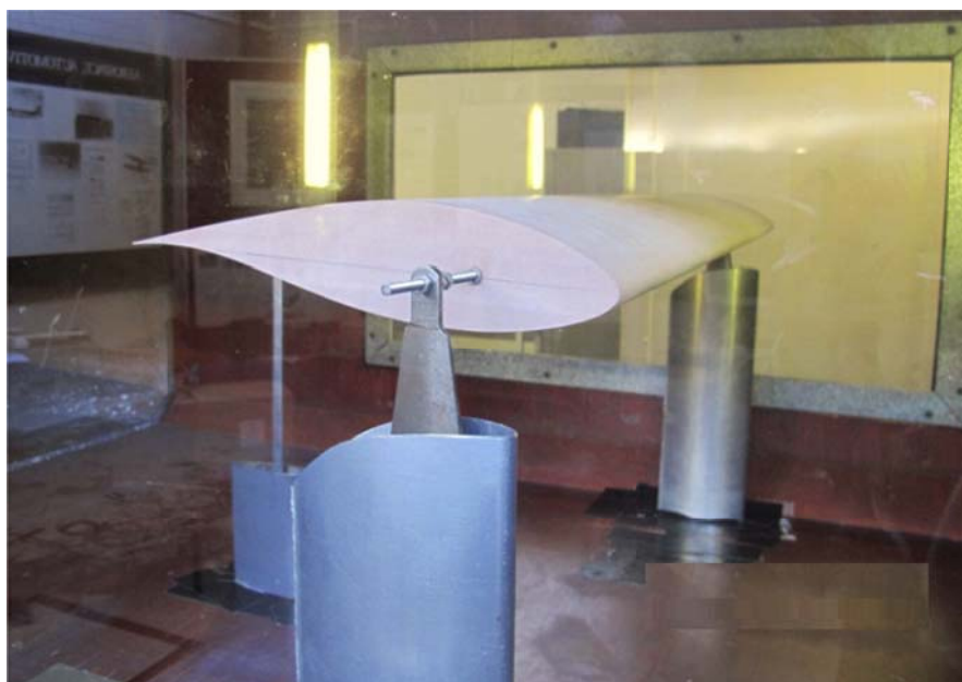
Figure 6-2 Wind tunnel test facility and mounting scheme
