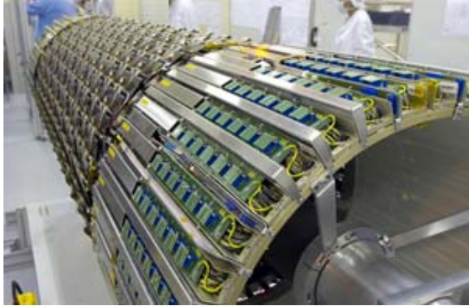
Figure 3.9: View of the silicon microstrips of the semiconductor tracker detector (SCT).
