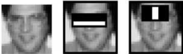
Figure 2. Haar-like features are extracted from sub-windows for face detection [22]
