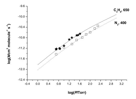
**Figure 10.** RRKM model (log ( $A/s^{-1}$ ) = 16.0) fits to the pressure dependence for SiH<sub>2</sub> + MeOH. Data points:  $\bigstar$ , C<sub>3</sub>H<sub>8</sub>;  $\Box$ , N<sub>2</sub>. Lines and step sizes indicated.
