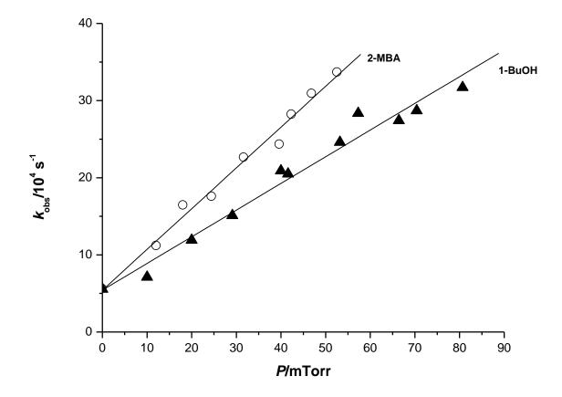
**Figure 4**. Second order plot for the reactions of  $SiH_2$  with 1-BuOH and 2-MBA at 10 Torr total pressure (added  $SF_6$ ) at 297 K.
