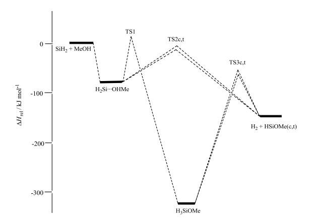
Figure 7. Potential energy (enthalpy) surface for the reaction of  $SiH_2$  + MeOH. All enthalpies are calculated at the G3 level.
