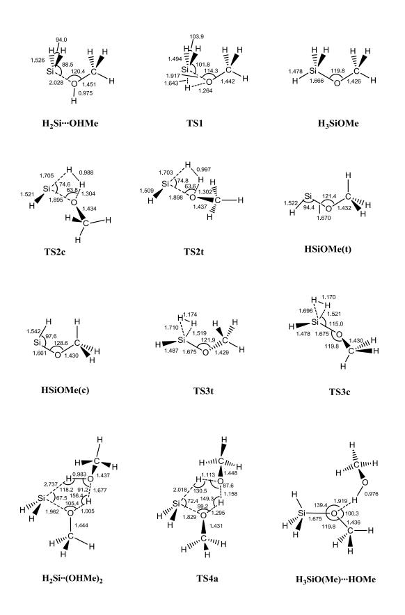
**Figure 6.** Ab initio calculated (G3 level) geometries of local minima and transition states on the energy surfaces of the  $SiH_2$  + MeOH and  $SiH_2$  + 2MeOH reactions. Selected distances are given in Å, and angles are in degrees.
