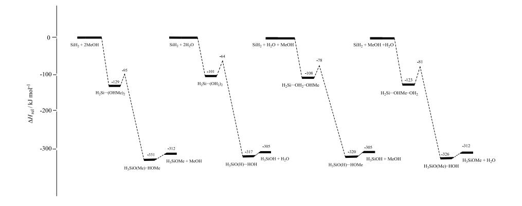
Figure 11. Comparison of PE surface (G3 level) for  $SiH_2 + 2MeOH$  with those for  $SiH_2 + 2H_2O$  and  $SiH_2 + MeOH + H_2O$ .
