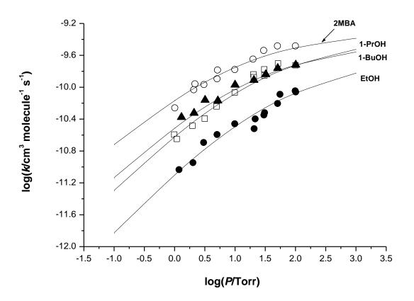
**Figure 5.** Pressure dependences for the second order rate constants for SiH<sub>2</sub> + ROH: •, EtOH;  $\Box$ , 1-PrOH;  $\blacktriangle$ , 1-BuOH;  $\circ$ , 2-MBA. Lines are RRKM theory best fits (see text).
