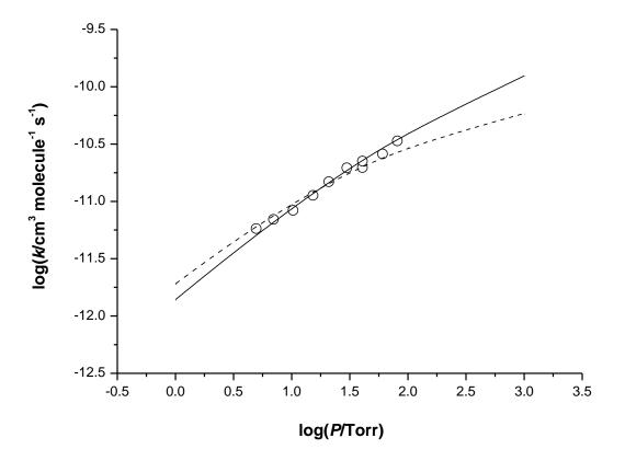
**Figure 8.** RRKM model fits to the pressure dependence for SiH<sub>2</sub> + MeOH (in SF<sub>6</sub>). Models: ---, log ( $A/s^{-1}$ ) = 16.0; ----, log ( $A/s^{-1}$ ) = 15.0)
