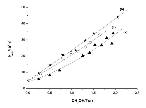
**Figure 1.** Second order rate plots for the reaction of  $SiH_2$  + MeOH at 297 K under various conditions:  $\blacktriangle$ , no buffer gas;  $\bigstar$ , 5 Torr total pressure (made up with SF<sub>6</sub>);  $\circ$ , 2 Torr added SF<sub>6</sub>. Lines are LSQ best fits: (a) and (c) quadratic; (b) linear.
