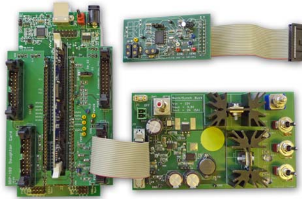
Fig. 7. Peak current mode Buck converter with 16W load (bottom right), analog control board (top right) and digital control board (left).
