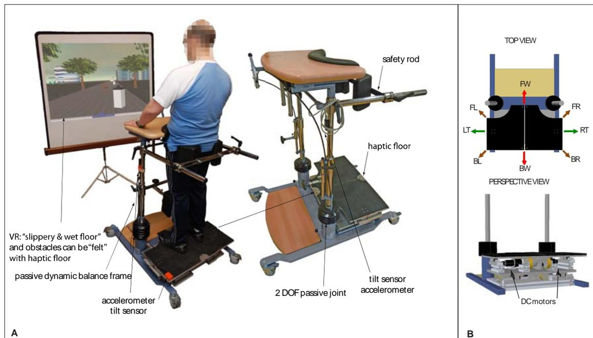
**Figure 1.** Haptic floor enables better interaction with task for virtual reality supported balance training (Cikajlo et al, 2011). At collision with the virtual object or on slippery floor (A) the haptic plates suddenly moves in the opposite direction, generating a postural perturbation (B).
