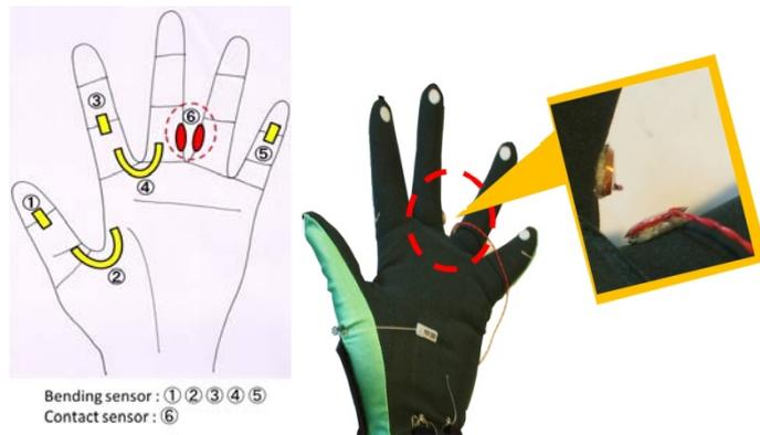
**Figure 3.** Sensor Layout(left) and the prototype(right).
