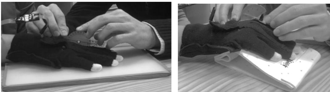
**Figure 4.** Examples of positioning templates and goniometric measurement
