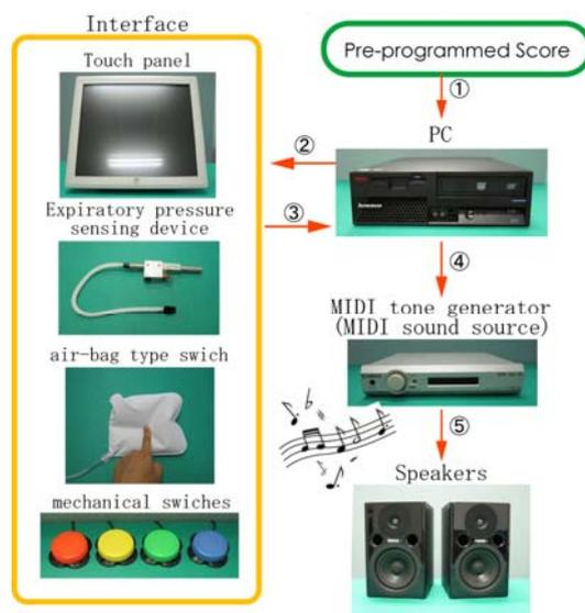
**Figure 1.** System structure of Cymis (Cyber Musical Instrument with Score.)
