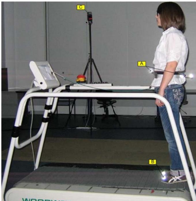
**Figure 1.** A participant using the RTSCA. A: pelvis cluster – a sprung loaded frame with 3-point contact to calculate the origin of the pelvis segment; B: markers on feet; C: one of the eight motion capture cameras used.
