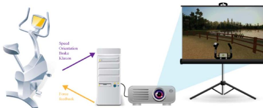
**Figure 2.** Instrumentation of the “Balade à l’EHPAD” application. The application is made of a bicycle simulator interfaced with the computer running the VR-based application. The environment is displayed by a beamer on a 78” screen.
