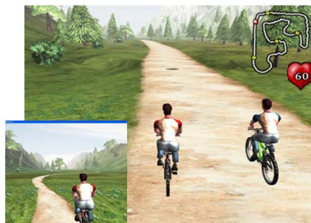
**Figure 2.** *Virtual Environment: Rider in red (insert figure on left) uses exercise intensity based on his measured heartrate to catch the pacer (in blue) who is far ahead. At the start the rider and pacer are together, the rider's trajectory in the VE is displayed in the right upper corner.*
