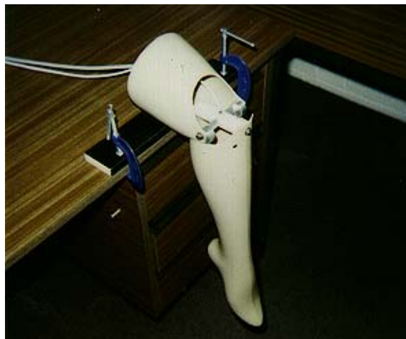
Figure 4. The artificial leg, showing hinge mechanism and entry point
