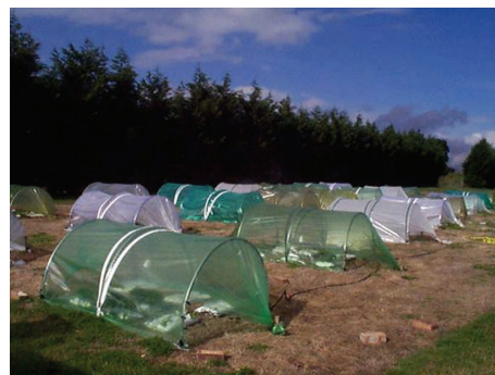
FIGURE 5: Horticultural tunnels undergoing field trials at the University of Reading; the light purple colored films contain stabilized optical brighteners.
