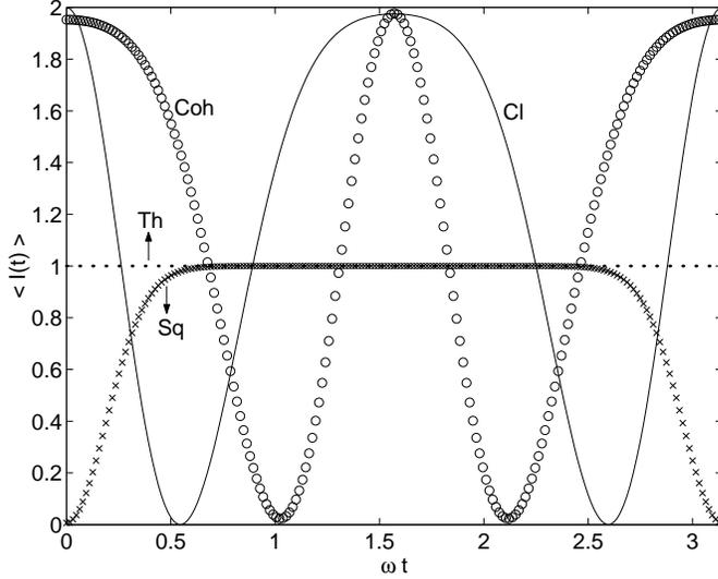
Figure 1.  $\langle I(t) \rangle$  as a function of  $\omega t$  for  $\omega = 10^{-4}$ ,  $\langle N \rangle = 200$ ,  $r = 6.4$ . We use units where  $\hbar = k_B = c = 1$ . Continuous line represents the case of irradiation with classical microwaves; line of circles, coherent states; line of crosses, squeezed states; and dotted line, thermal states.
