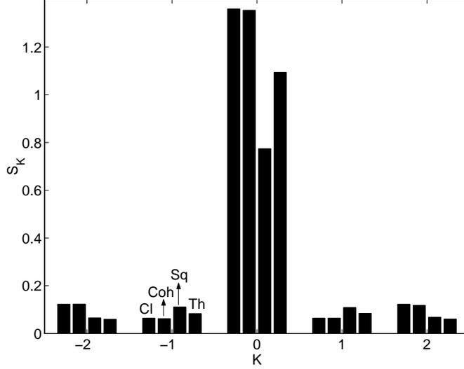
Figure 3.  $S_K$  coefficients for the electrons with  $\langle N \rangle = 200$ ,  $r = 6.4$ . We use units where  $\hbar = k_B = c = 1$ . The bars correspond to irradiation of the ring by (from left to right): classical, coherent, squeezed, and thermal states.
