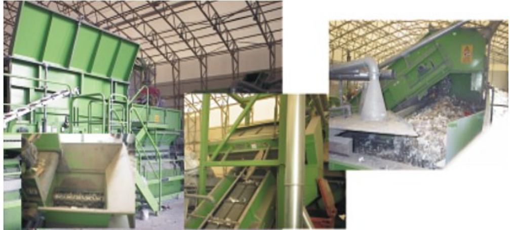
Figure 7. Processing of commercial waste: shredder, magnet and Eddy Current.
