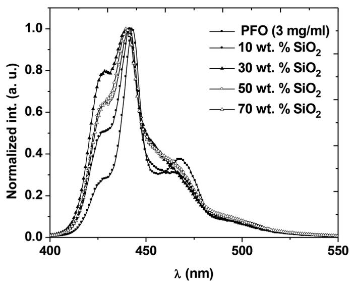
FIGURE 6. Normalized fluorescence intensity of pure PFO and PFO/SiO<sub>2</sub> nanocomposite
