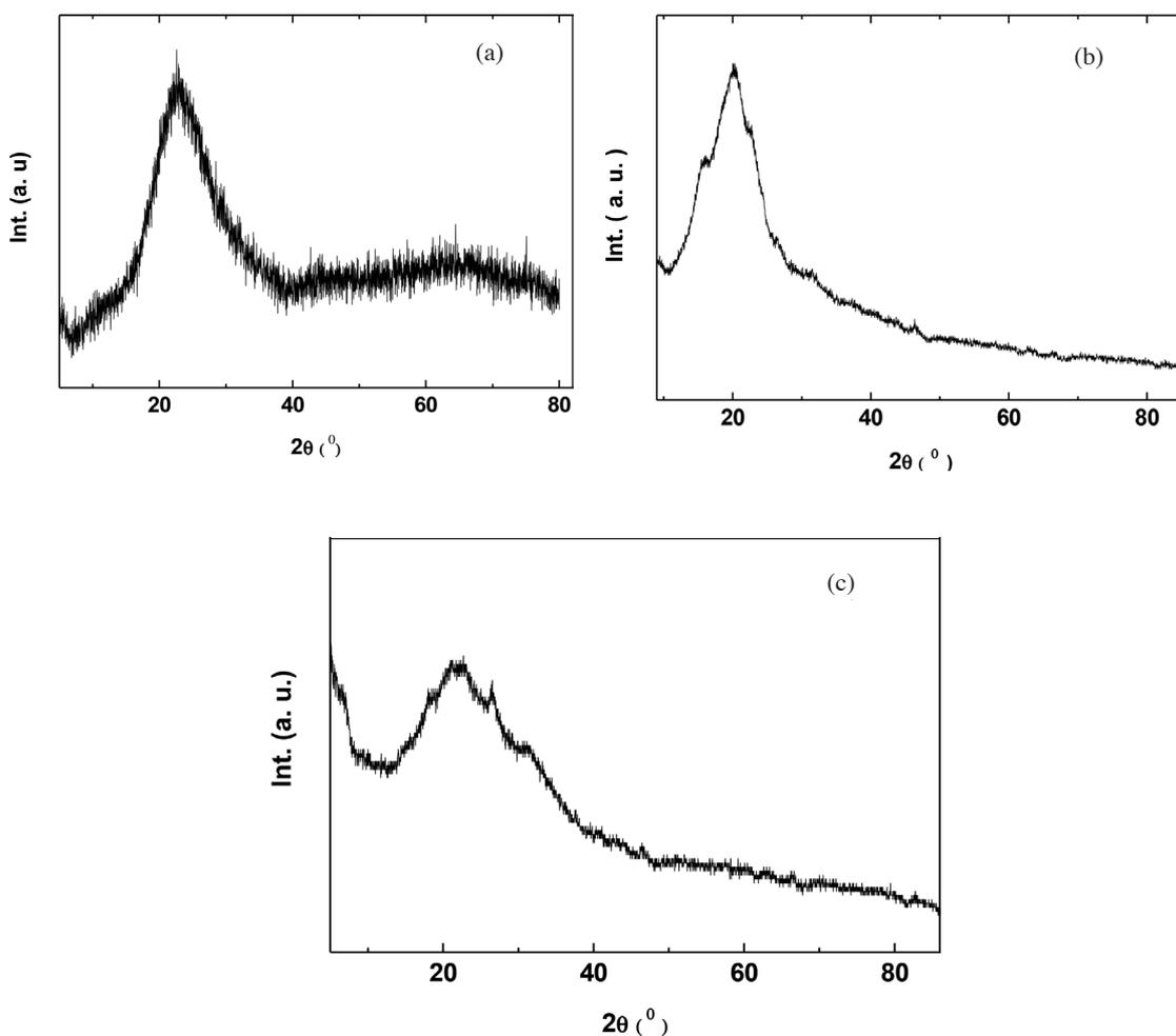
FIGURE 1. Typical XRD patterns for (a) SiO<sub>2</sub> NPs, (b) Pure PFO and (c) PFO/50 wt.% SiO<sub>2</sub> NPs
