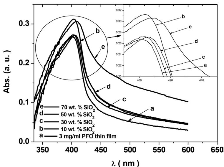
FIGURE 3. Absorption spectra for PFO and PFO/SiO<sub>2</sub> nanocomposites
