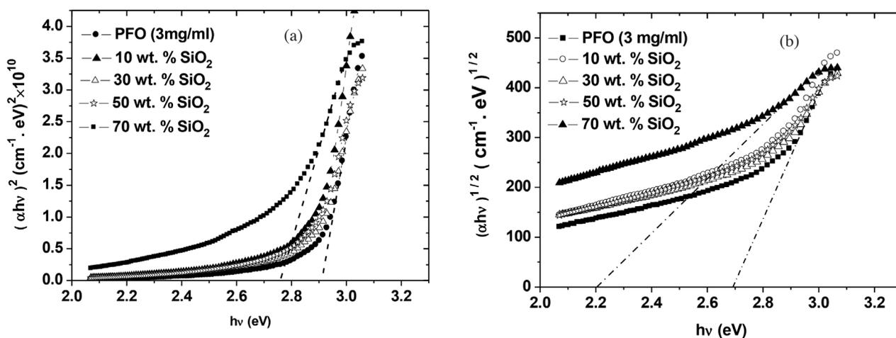
FIGURE 4. Dependence of (a):  $(\alpha hv)^2$  and (b):  $(\alpha hv)^{1/2}$  on photon energy ( $h\nu$ ) for Pure PFO and PFO/SiO<sub>2</sub> nanocomposites
