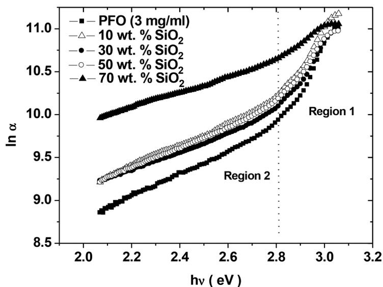
FIGURE 5.  $\ln \alpha$  as a function of photon energy for PFO and PFO/SiO<sub>2</sub> nanocomposites
