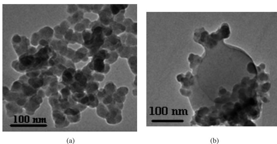
FIGURE 2. TEM images of (a) SiO<sub>2</sub> NPs (b) PFO/SiO<sub>2</sub> nanocomposite (50 wt. % SiO<sub>2</sub>)
