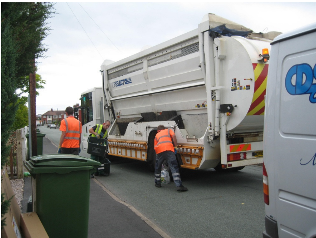
Image 3: Two stream partially co-mingled systems are where residents are required to separate materials into two categories, usually fibres (paper/ card) and containers (glass, cans and plastic bottles). Separate containers are provided for each category the contents of which are loaded into separate compartments on a twin compartment collection vehicle.
