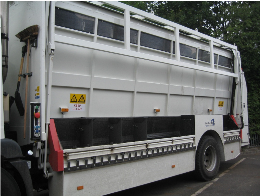
Image 1: Kerbside sort systems are where materials are sorted by material type at the kerbside into different compartments of a collection vehicle.
