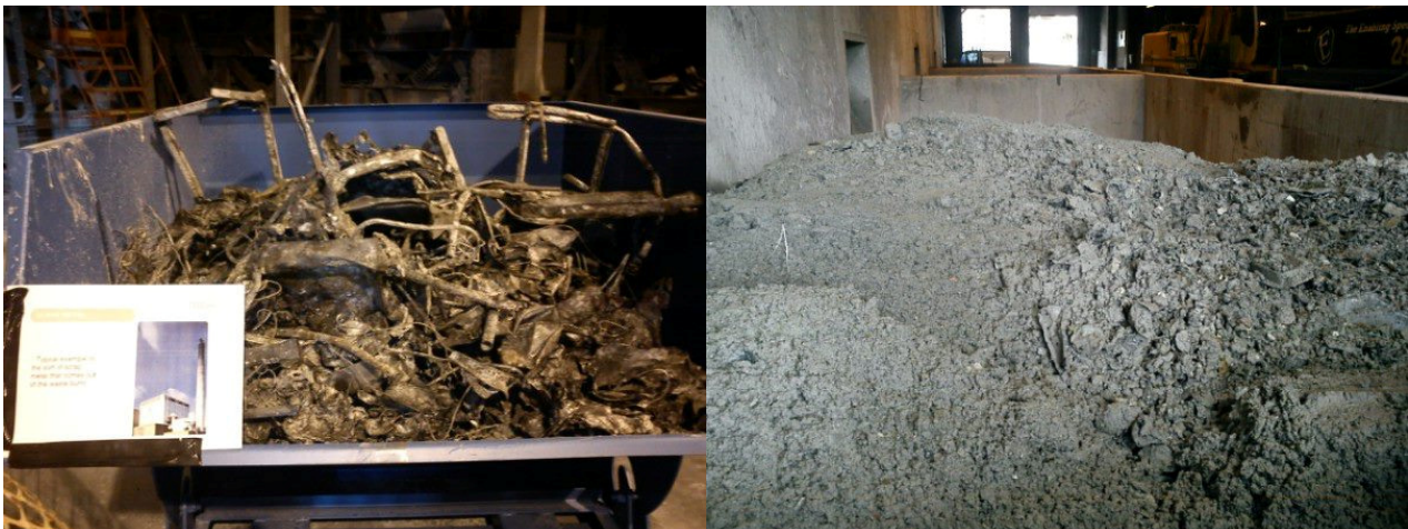
Image 8: Metals and ash from the back-end of the incineration plant
