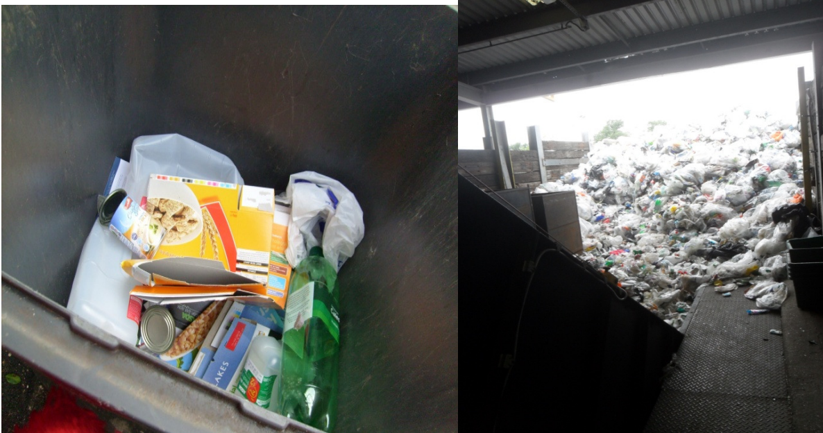
Image 2: Single stream co-mingled systems are where materials are collected in a single compartment vehicle with the sorting of the materials occurring at a MRF (Materials Recovery Facility).
