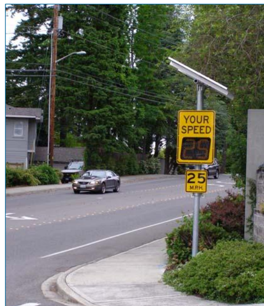
Figure 37. DSFS system in Bellevue, Washington (City of Bellevue 2009)
