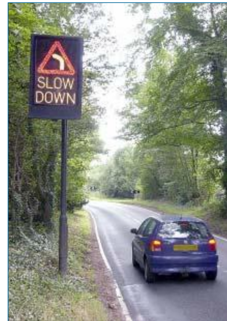
Figure 36. DSFS system in Norfolk, Virginia (Winnett and Wheeler 2002)
