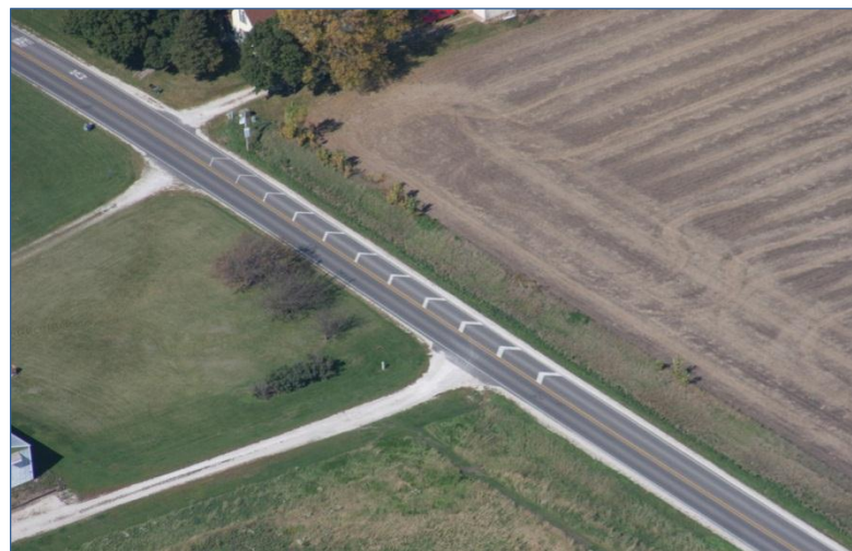
Figure 13. Converging chevrons at entrance to small rural community (Hallmark et al. 2007)
