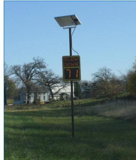
Dynamic speed feedback sign
