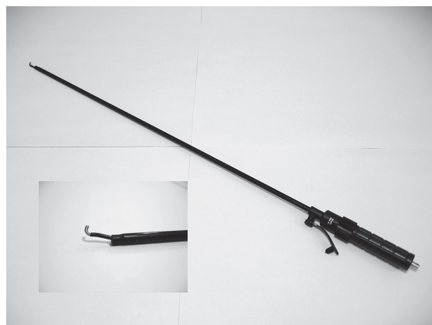
Fig. 2 An articulating hook cautery (Karl Storz, Tuttlingen, Germany). The hook cautery has a long body (46 cm), and the connecting jack is located behind the body. It is used with its tip set at a 15° angle.
