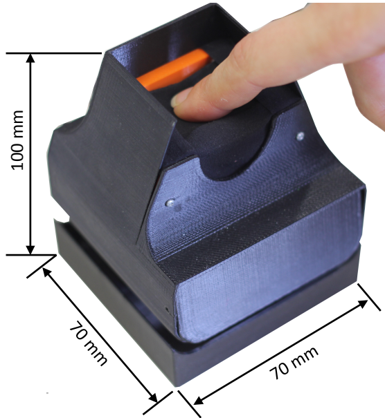
Figure 5.1: A subject's finger interacting with FYD-2. The dimensions of the device are also reported.
