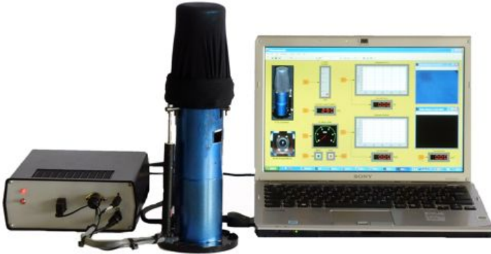
Figure 4.1: The system FYD: starting from the left side, it is possible to see the electronic box, which contains the motor driver and the DAQ card, the FYD prototype and a computer to control the system.
