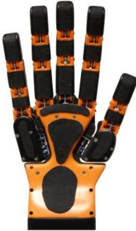
Figure 1.1: THE first Hand prototype: a 5 fingers, 16 DoFs robotic hand driven by tendons.
