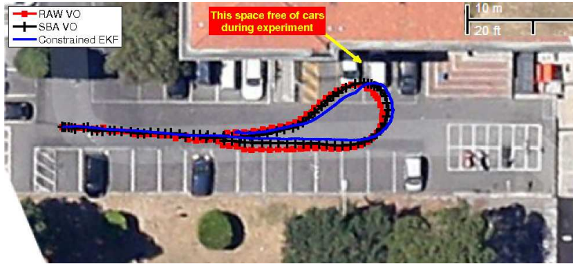
Figure 6.4: Comparison of the reconstructed path by using the proposed approach (Constrained EKF – blue line), raw visual odometry (RAW VO – red-square line) and visual odometry with multi-frames sparse bundle adjustment refinement (SBA VO – black-cross line).
