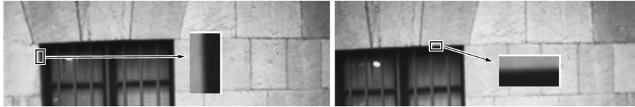
Figure 5.2: Example of a possible matching ambiguity connected with the use of covariant feature detectors (e.g., SIFT).
