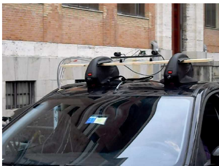
Figure 6.8: Navigation sensors suite mounted on the top of the car used for city experiments.
