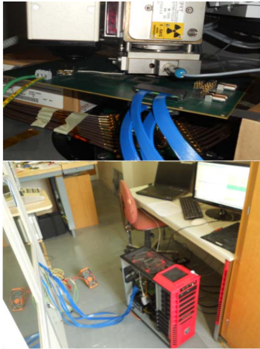
Fig. 42. Test setup used during the irradiation test, performed at the CERN 10-keV X-ray facility.
