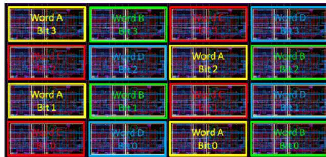
Fig. 34. Spatial interleaving of the storage elements in the FIFO array, foreseen in the upgrade of the radiation hardened module.
