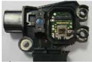
Fig. 47. Valeo mechatronic 3 rd generation brush-holder (BH03G) regulator System on Chip (SoC). The IC is mounted on the leadframe without package.
