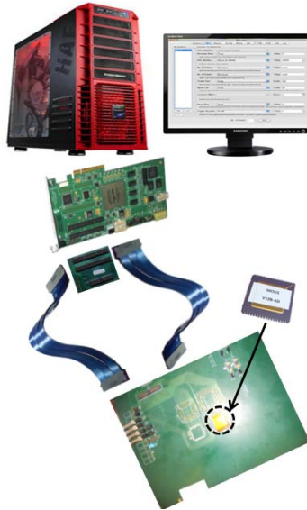
Fig. 37. Test-bed employed in the characterization of the test-chip FF-TC1.
