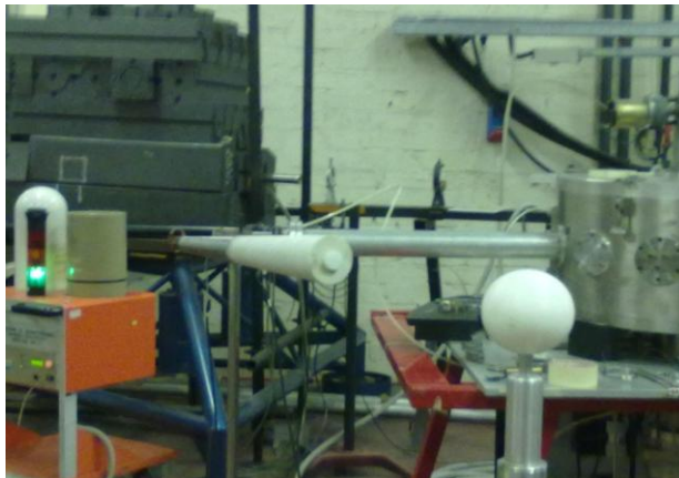
Figure 6.4: The 5 in. Bonner sphere and shadow cone II positioned in the CN accelerator room of the INFN-LNL (120° angle). The Be accelerator target is on the left side of the picture.
