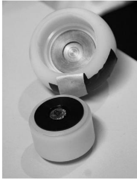
Figure 2.1: PE-insert, the gold foil was placed with and without a Cd shield inside 2.5 in. Bonner sphere (Garny, 2011).
