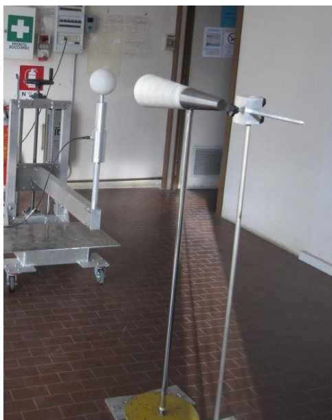
Figure 5.9: shadow cone II positioned between 5 in. Bonner sphere and an ^{241}\text{Am} –Be neutron source which is visible on the right side of the picture.
