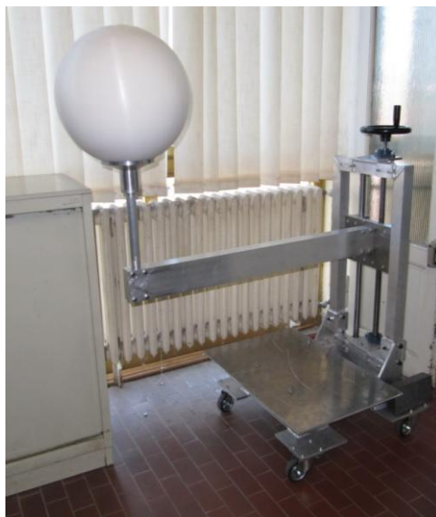
Figure 5.4: View of the inch holder for the Bonner spheres manufactured at DICl.
