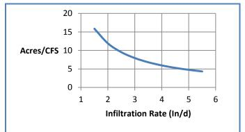
Figure 3. At the long-term infiltration rates of 2 - 2.5 in/d measured in this study, approximately 10 acres are required to infiltrate 1 CFS. That relationship corresponds to pumping water at 3,500 gpm onto a 70 acre field.
