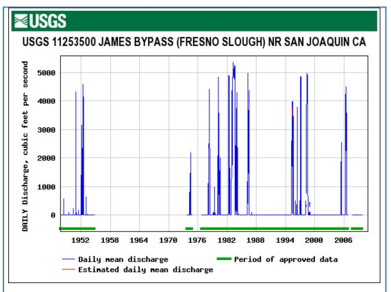
Figure 1. Flood flows past the James Weir have a reoccurrence interval of 2 – 3 years and vary greatly in magnitude, at times exceeding 4750 CFS system design.
