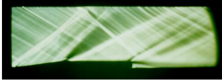
Fig. 13. Flow past a half wedge strut, parallel liquid injection, M=2, P 0j /p a = 20
