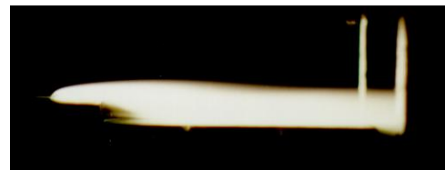
Fig. 10. Transverse liquid injection ahead of step; M=2 , P_{oj}/p_a = 20 , d_j= 1.2 mm
