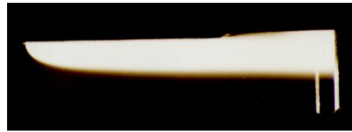
Fig. 9. Transverse liquid jet from a plain wall ; M=2 , P_{oj}/p_a = 20 , d_j=1.2 mm
