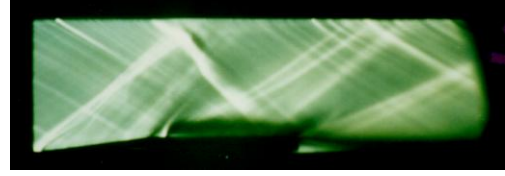
Fig. 15. Flow past a half wedge strut, parallel/transverse liquid injection; M=2, P 0jv /p a = 20, P 0jh /p a = 14.
