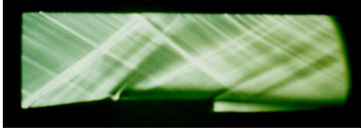
Fig. 14. Flow past a half wedge strut, transverse liquid injection; M=2, P 0j /p a = 20,
