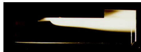
Fig. 11. Transverse liquid jet behind a step; M=2 , P_{oj}/p_a = 20 , d_j= 1.2 mm
