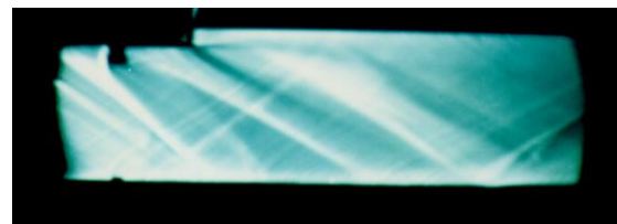
Fig. 7. Flow past a backward step, cylindrical protuberance, M=2 ; h, H = 5.7, 5.7 mm
