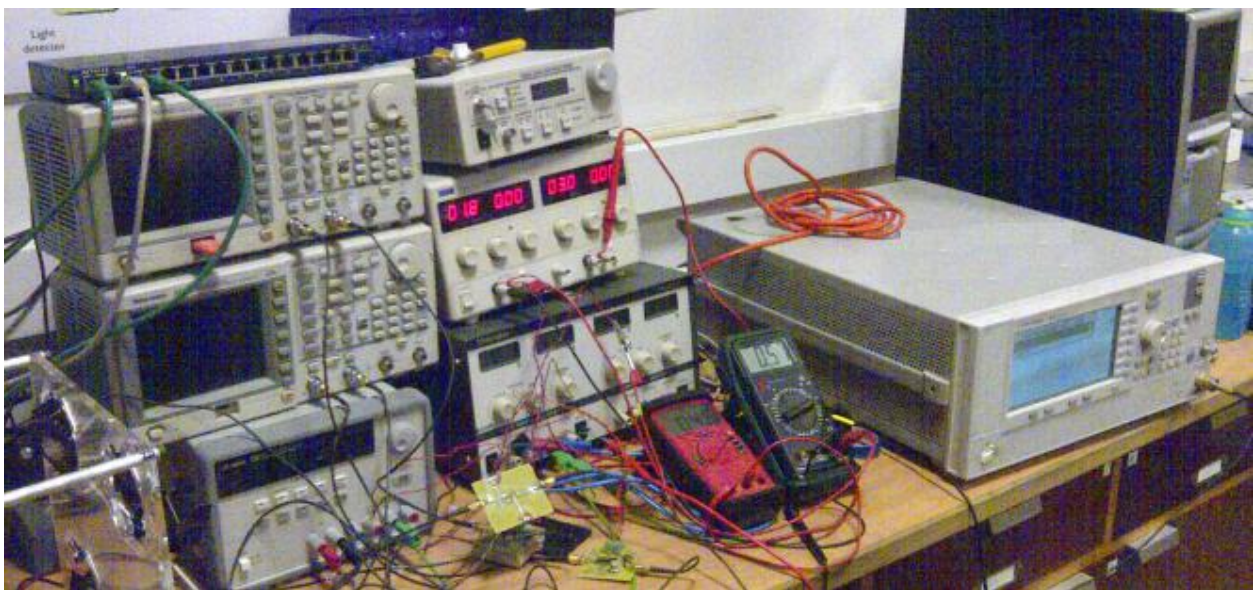
Figure 6.23: A typical measurement setup for the power amplifier
