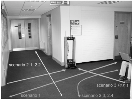
Fig. 3. Environment of the first experiment. The movements of the three scenarios are shown by the arrows. Scenario 1 corresponds to the subject moving from “right to left” and “left to right” in front of the robot. Scenario 2.1 and 2.2 have the subject moving past the robot on its right side from front to back and visa versa. Scenario 2.3 has the subject moving along a curved path from the robot’s front to the passage at the robot’s left. Scenario 2.4 is the same but with the subject moving in the opposite direction. Scenario 3 corresponds to the subject moving “forward” in a straight line from anywhere within a semi-circle ahead of the robot, stopping in front of the robot.
