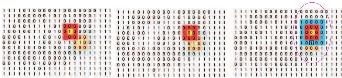
Figure 2: Influence area of pixel (7, 16) when it is equal to 1.
