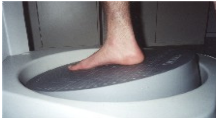
Figure 1. The platform of the Biodex stability system.
