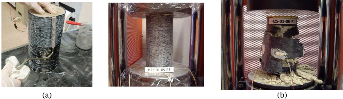
Figure 11: (a) CFRP confinement preparation. (b) Specimen prepared to be preloaded at 85% of maximum load capacity. (c) Specimen broken with a preload of 65% of the maximum load capacity.
