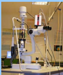
FIG. 1. Slit-lamp and digital video camera used to capture the images of frontal cornea.
