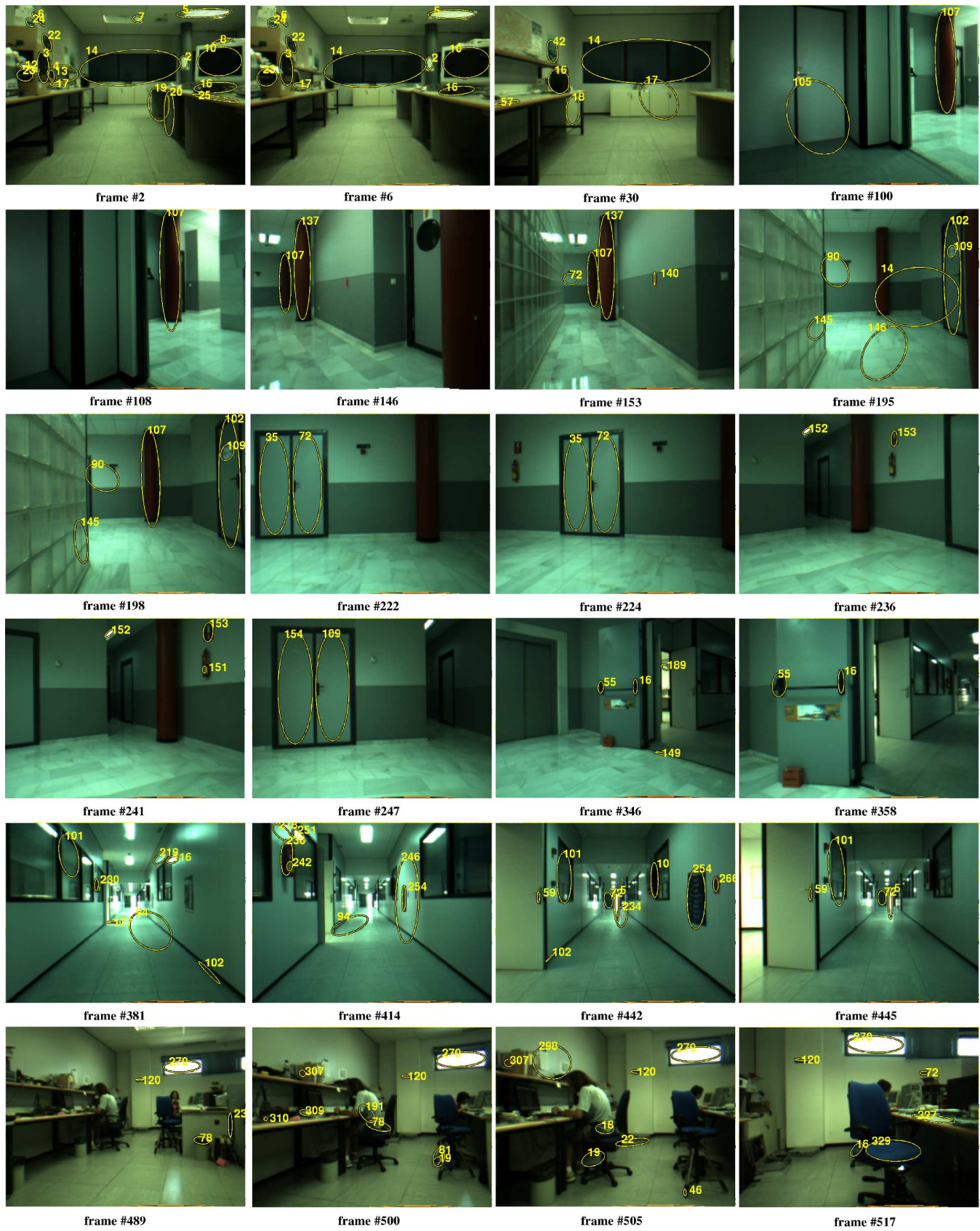
Fig. 11. Experiment in an indoor environment. Detected regions were matched during the trajectory using a nearest neighbour algorithm. It can be seen how corresponding regions are matched when the same scene is observed, e.g. in the following frame sets: (#2, #6, #30), (#100, #108), (#146, #153, #198), (#222, #224), (#236, #241), (#346, #358), (#414, #442, #445) and (#489, #500, #505, #517)
