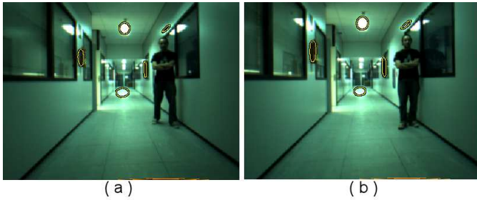
Fig. 2. a-b) Regions generated by the proposed detector on two images taken from a mobile robot. Representing ellipses have been chosen to have the same first and second moments as the originally arbitrarily shaped region (see Fig. 11 for more examples).
