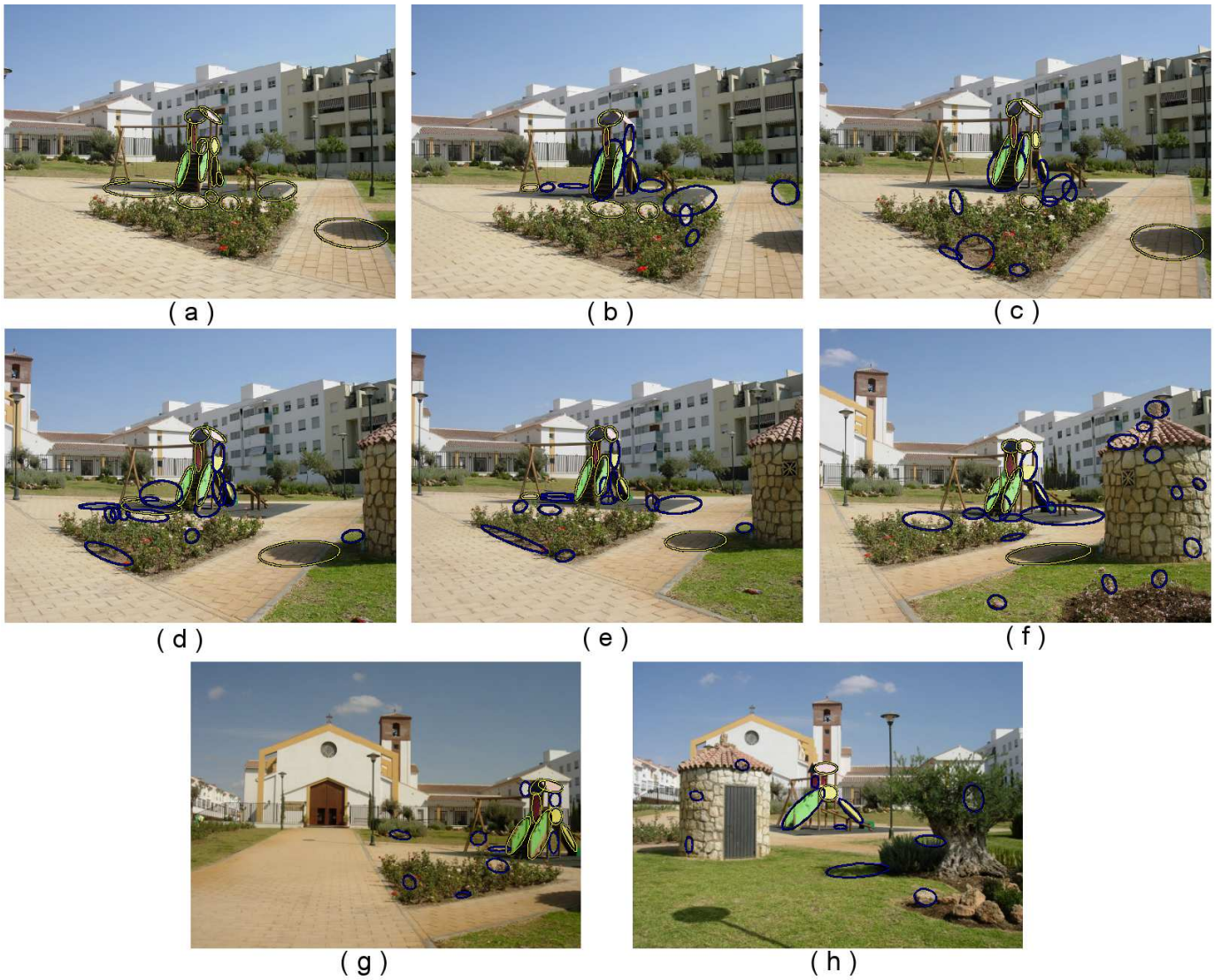
Fig. 5. a) Reference image and detected features;b)–h) images matched against the reference image. The colour of the ellipses determines if the associated region has been matched to a reference feature (displayed in yellow) or not (displayed in blue).
