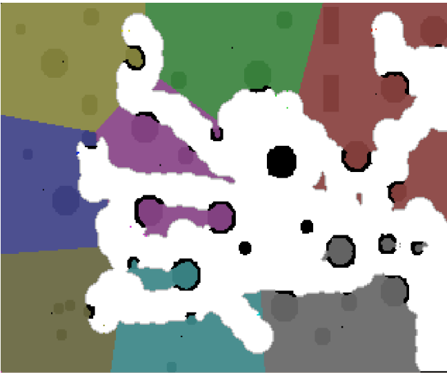
Fig. 2. The same exploration method as in Fig. 1. applied to an unstructured working space populated with scattered obstacles. Each region is assigned to a single robot ( K = 8 ). The black areas are already-found obstacles and the irregular spots and rectangles in the background are obstacles that have not been found yet.
