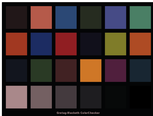
Color Plate 4. Top: Color stimuli of the ColorChecker Chart under fluorescent light source (DAY lamp). Bottom: Simulation of the image captured by our digital image capture device. (Francisco Martínez-Verdú, et al, pp.279–295).
