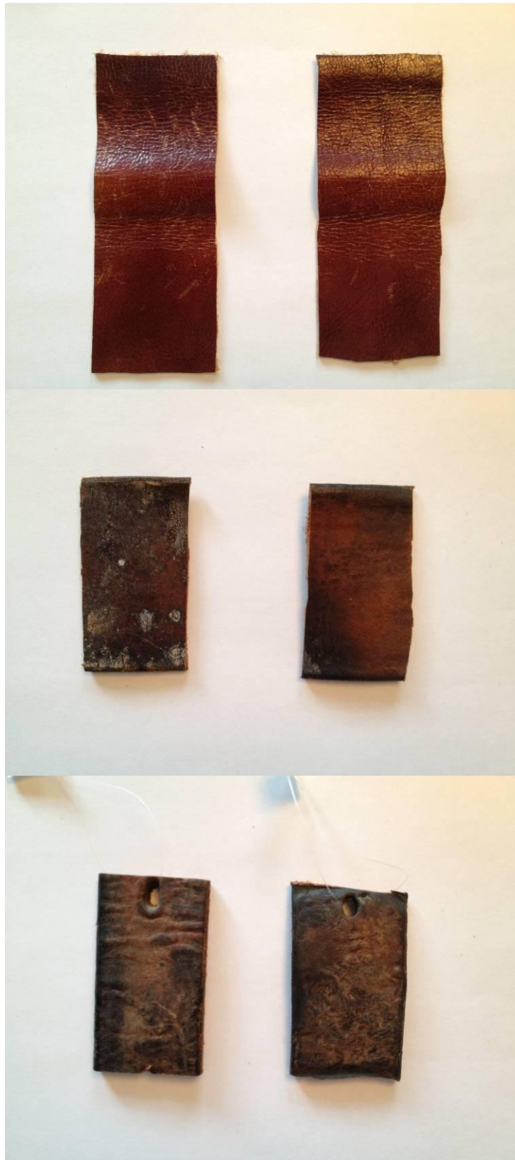
Figure 8. British Museum Leather Dressing: Control samples and post treatment. Samples to the left are control samples. Top: type 1, middle: type 2, bottom: type 3. Photo: Lena Ludwick 2012
