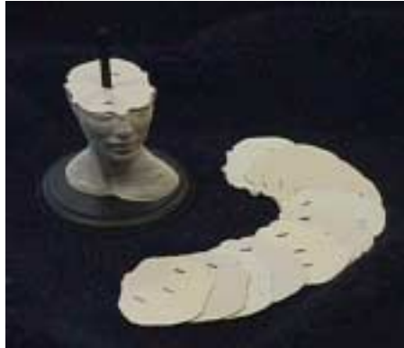
Figure 7: A 3D Puzzle: the concept of layered manufacture.
