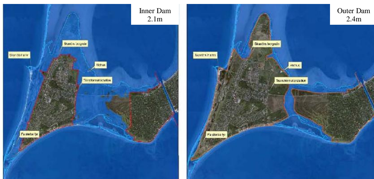
Figure 4.3.2.4 Proposed inner and outer dam with different water levels
